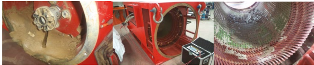
Our field failure detection field service is winding damage occurred at 19 MVA generators due to water cooler puncture.
