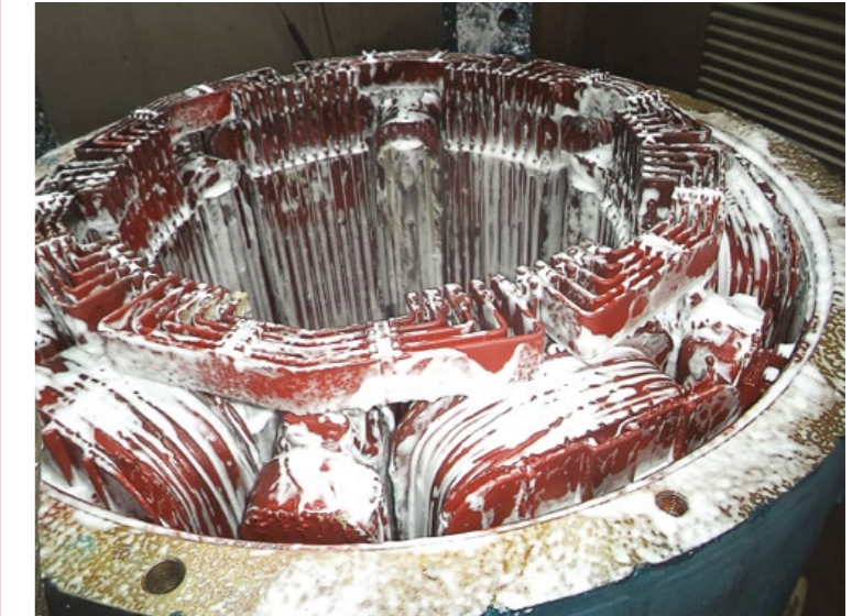
1500 Hp DC mixer motor maintenance.
