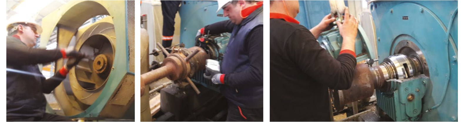
Shifting bed replacement and laser coupler adjustment of 2500 kW Atlas Copco compressor motor.
