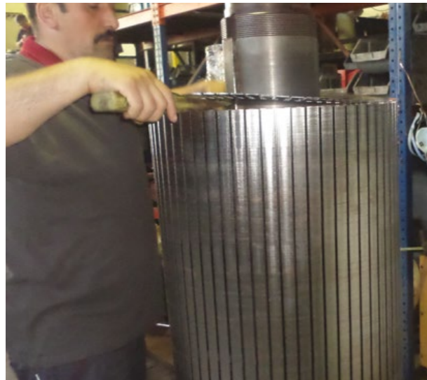
1475 kW Pump motor rotor core manufacture and rewinding.
