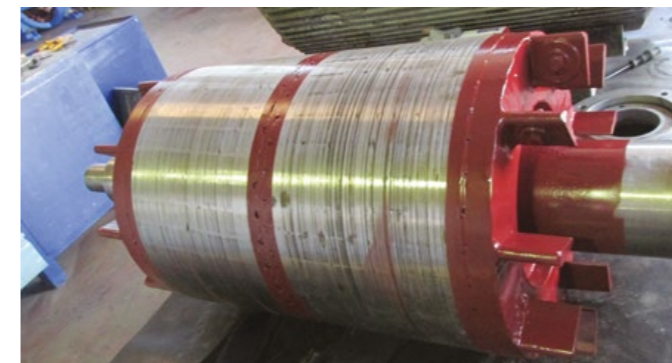
181 kW Atlas Copco compressor Siemens brand motor winding, double lobe rotor winding.
