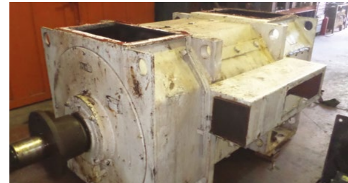
Our 735 kW DC pump motor, workshop and field service maintenance and repair work.
